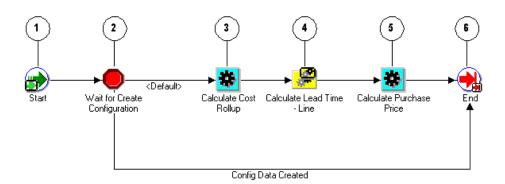
The Create Manufacturing Configuration Data - Line, Manual begins after Line Flow - Configuration or Line Flow - Configuration with Authorize to Ship (RLM) is selected as the appropriate line flow for the order line. The Create Manufacturing Configuration Data - Line, Manual process is initiated as a subprocess of the selected line flow.
